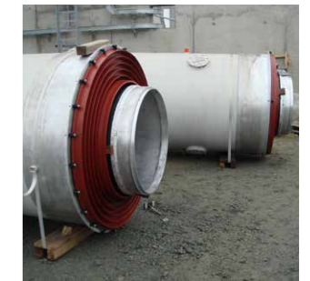
4 Watertight connection to generator.
